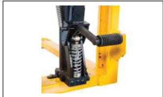
Effortless and quick lifting for using foot pedal without loads
