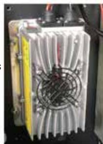
For PSExxB SL the charger with current 12A is used. The standard charging time is 7 hours.
