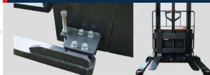
The support legs are fixed with screws located outside of the truck's body (4 screws for each side). The position can be easily adjusted according to the customer's needs to achieve the overall width of the truck:
