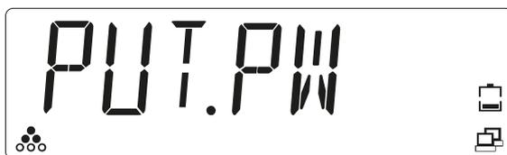
5. Place the number of parts (reference quantity, in this example 20) on the load plate.
