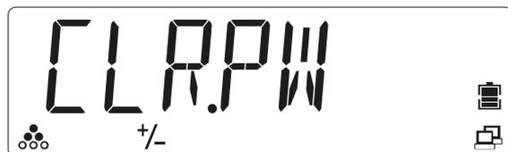
2. Press the
