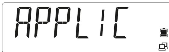
Selection of the procedure for the configuration of the A/D converter:
