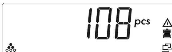
9. To count parts that are removed from a container, after initializing the sample weight, place the container with the items to be counted on the scale and press the  $\rightarrow T \leftarrow$  (Tare) key.
