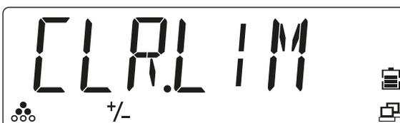
If there is no reference sample weight on the load plate or the weight is less than 2 d, [REF.ERR] (reference error) is briefly displayed in the display. Apply higher sample weights.
