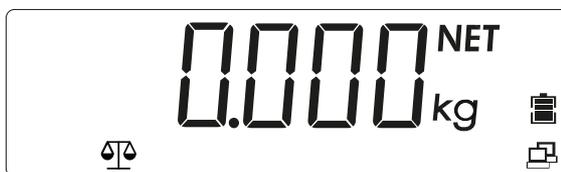
The scale has been tared. The tare weight remains saved until it is deleted or overwritten with a new weight.
