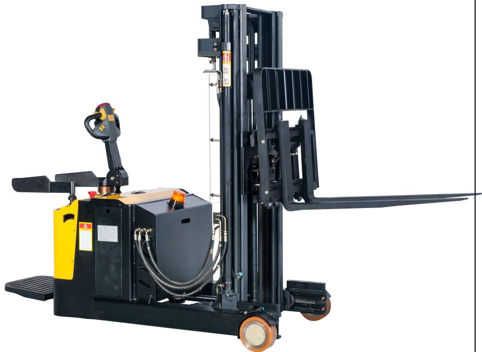
**Mast Reach stacker is the perfect selection that combines the counterbalance stacker with the reach-mast, where a short length is needed with a higher lift capacity required.**
